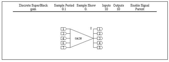
**Figure 6-1.** Poorly Connected Gain Block
